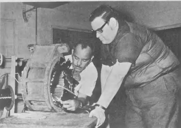
Robert van der Schoot, UTS student, watches attentively as Everaldo Everon of Mechanical-Electric Shop rewinds motor. Robert van der Schoot, estudiante di UTS, ta mira cu atencion com Everaldo Everon di Mechanical-Electric Shop ta pasa waya nobo na un motor.
